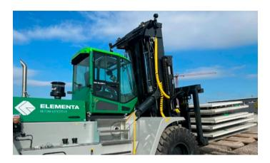
It also includes a range of features such as individual fork positioning, auto engine, lighting and ignition shutdown, and a height indicator laser, as well as the latest fuel-efficient engine for less exhaust emissions, compliance with tough EU environmental regulations, and reduced noise.
